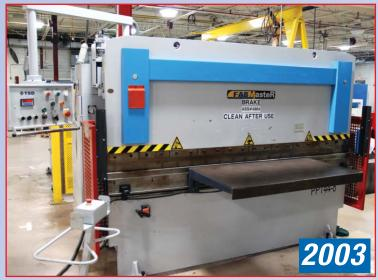
FABMASTER 8' X 44 TON HYD, PRESS BRAKE
